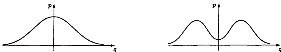
Fig. 8. Different distributions p of the inversion coordinate q in an ammoniatype molecule, referring to different decompositions of the same thermal nonpure state into pure states. This figure refers to some fixed inverse temperature. The figure corresponds to fig. 4 and is not based on a calculation. For chiral molecules, the value p(q = 0) is expected to be very low.
